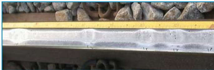
Squats: V-shaped or half-moon-shaped hollows, especially from heavy haul traffic. Tears are growing beneath the surface
